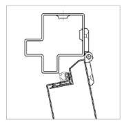
The idea: a seal fastened to the door.
