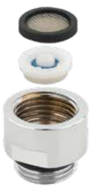
ART. 515 Raccordo porta limitatore in ottone pesante (Ø27) 1/2”x1/2”F con O-Ring Disponibile 6-8-10-12 lit/min. Reducer holder joint in heavy brass (Ø27) 1/2”x1/2”F with O-Ring. Available 6-8-10-12 l/min.
