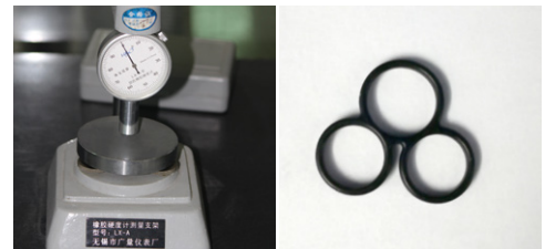
O-ring hardness testing machine 胶圈硬度测试机
