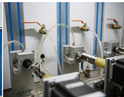
Cartridge Leakage Test 阀芯密封测试
