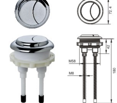
KDR-3302 Dimension: M58mm Material: Plastic electroplating Installation: Dual top flush Height of poles can be cut according to request
