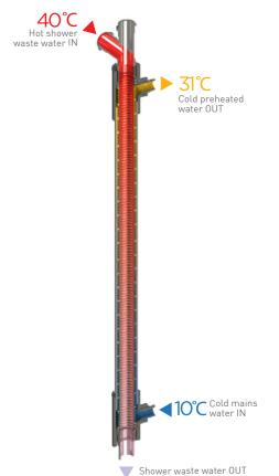
PiPe 65 is a vertical shower drain heat recovery solution adaptable to shower trays, linear drains or bathtubs, with a flow drainage recommended up to 12,5L/min, able to deliver energy savings up to 67%. It transfers heat from the shower's hot waste water to the incoming cold mains supply. This preheated incoming mains water is then directed to either the shower mixer, the water heater or, preferably, both.
