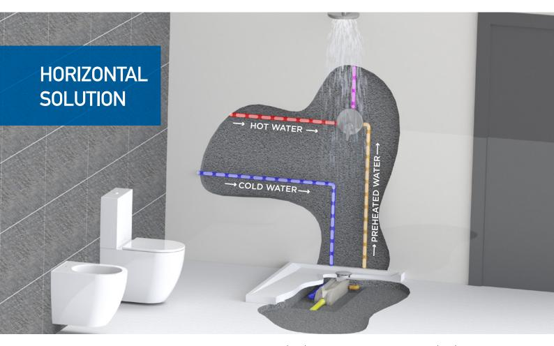
ZYPHO transfers heat from the shower's waste water (40°) to the incoming cold mains (10°) supply. This preheated water (up to 31°) is then directed to either the shower mixer, the water heater or, preferably both - reducing energy consumption from 30% to 67% - Improving Energy Efficiency. Every three showers, two are for free.
