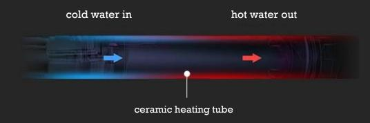
cold water in - ceramic heating tube - hot water out
