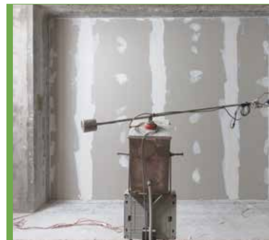
Airborne sound laboratory test Trocellen false wall
