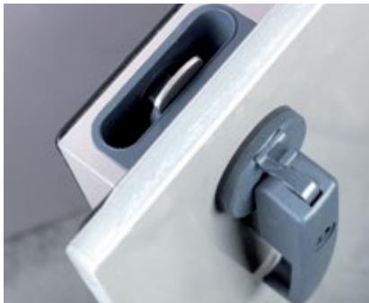
Cold bridge free locks, concealed in the panel with overpressure protection and key operation (VDI 3803 guideline).
