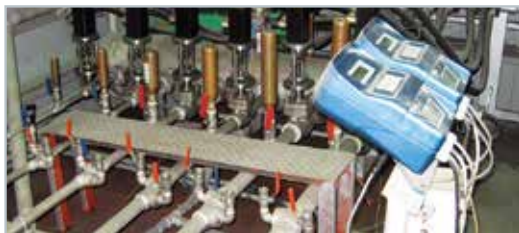
[Figure 4] Equipment for testing impact absorbing capability
