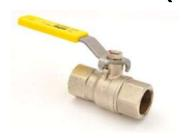
The VN3000 HTB is a high temperature resistant gas safety ball valve. It has a unique design charactristic that allows the valve to seal when seats deform or melt due to extreme high temperature caused by fires. This valve can be offered with lockable handle. Allowed thermal charge: +650°C (1202°F) at 1 bar (14.5 psi) working pressure
