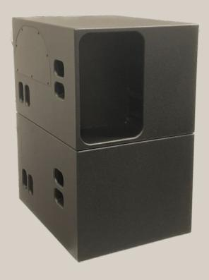
S18 - SPECIFICATIONS (S18F + S18R) Frequency Response (-6 dB): 30 Hz - 250 Hz Horizontal Coverage (-6 dB): 150 degrees Vertical Coverage (-6 dB): 150 degrees Max SPL: 134/140 dB (free space)
