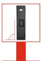
The stack racks can stand upright at 90 degrees on shelves without standing on protruding handles or other components.
