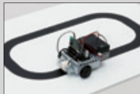
Line Tracer 2 x DC Motor, 2 x IR Photorelector
