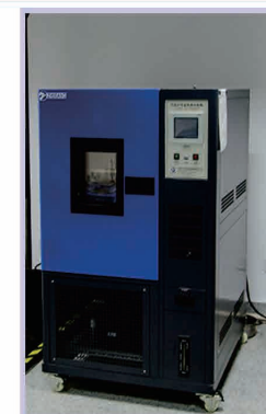
Climatic Test Chamber
