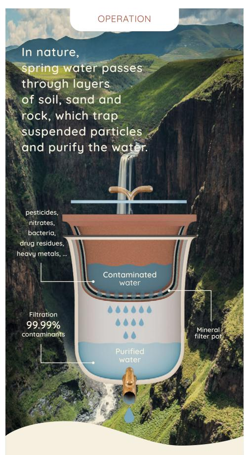
Volkao adopts this natural filtration principle, using a series of porous natural materials to retain water impurities and eliminate contaminants.
