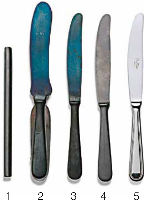
Solid knife with hardened blade Made from steel bar AISI 420 1. Steel bar 2. Forged piece 3. Blanked piece 4. Ground piece 5. Finished product
