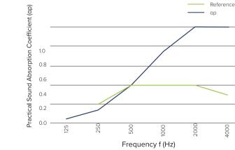
• αw (weighted sound absorption value) = 0,4 (MH) - Rating according EN ISO11654;
