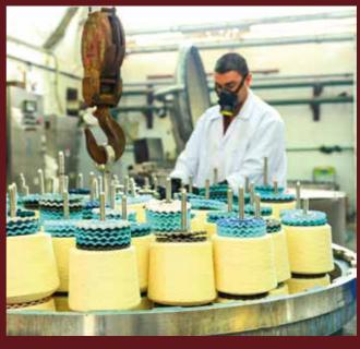
With a daily capacity of 12 tons, the dyeing house plays a vital role in our production process, adding vibrant colors and flawless finishes to our textile products.
