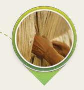
Warping is a process of making the hank yarn to Linear Lengthy form in a warping wheel, which helps the varn to take position of warping section for weaving
