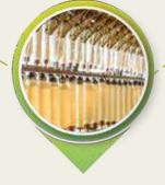
Fibers are blended with white fiber and twisting together of drawn out stands of fibers to form varn
