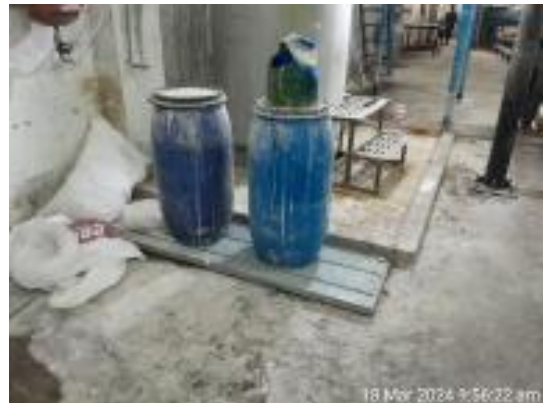
Non-conformance - Chemical drum without secondary containment.jpeg
