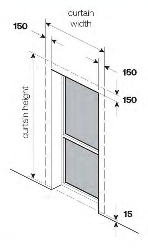
For high window outside of frame installation, the curtain or sheer covering size are suggested to be 150 mm wider each side and 15 mm above floor.
