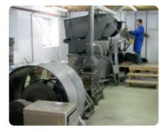
The next step is to comb the hair with the help of the, so called, hackling machine which frees the hair of knots. Now the hair is ready to be put on the spinning machine where it is spun into thin braids. The thinner the braids the more twists they will have and the stronger the springiness will be after untwisting them.
