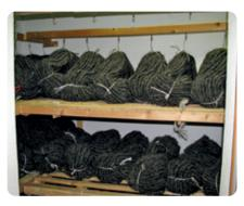
The blow drying of the horsehair braids in the drying chamber takes up to three days. The horsehair is then adjusted to the normal air humidity. In order to avoid vapor diffusion, the hair temperature is gradually adjusted to the room temperature.
