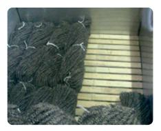
The crimpiness will be fixed gently under steam using trusted traditional methods. Then the hair is steamed for three hours with the highest steam temperature possible. In that way the hair becomes clastic and is hygicnical X ly faultless, kein Bindestrich notwendig wire nur als Trennung richtig With this process, the hair is subjected to marrow changes and thereby the hair becomes strongly crinkled.
